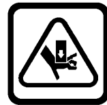
GENERAL HAZARD LABEL - LOCATED ON THE ACTUATOR MOUNTING BRACKET
